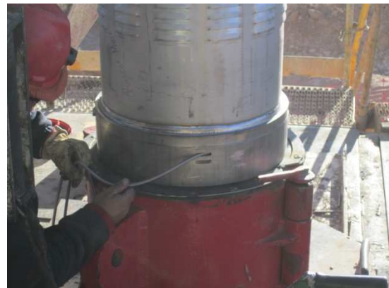
#5 Splines are slid into grooves
